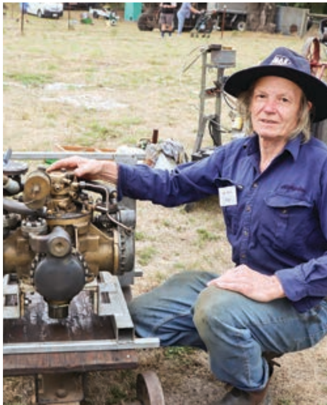
Warwick Bryce displayed his WWII torpedo engine which was powered by kerosene and used compressed air to enable it to run under water. A41_1223
