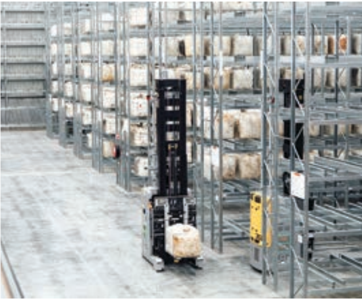
An AGV moves a wool bale at the Ravenhall centre.
