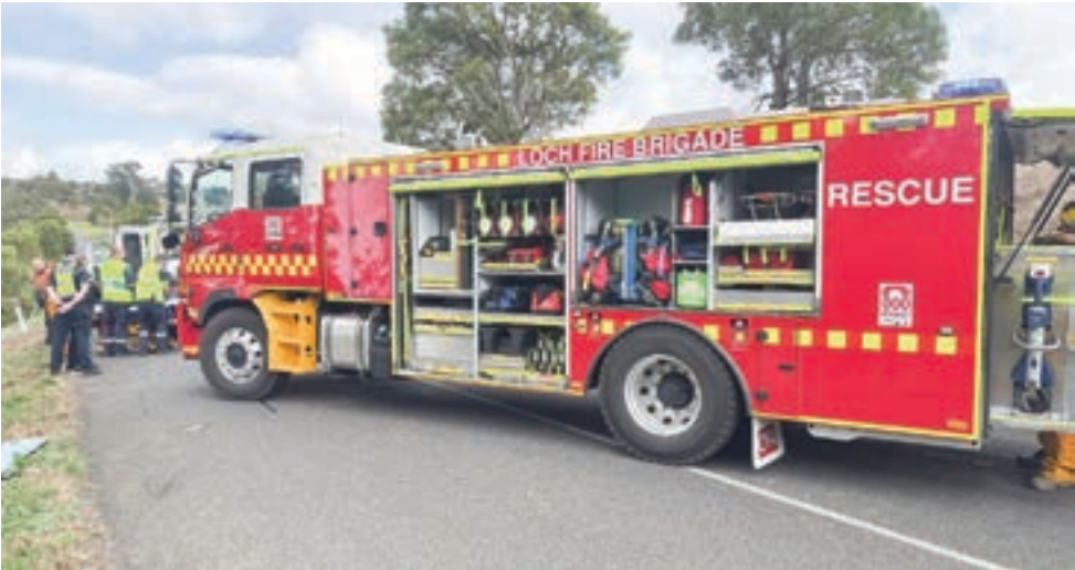
The new rescue truck for Loch CFA Fire and Rescue comes with emission free stowage, battery operated tools, increased capacity for heavy vehicle response with a rescue work platform and increased ability to carry a full steep angle cache.
