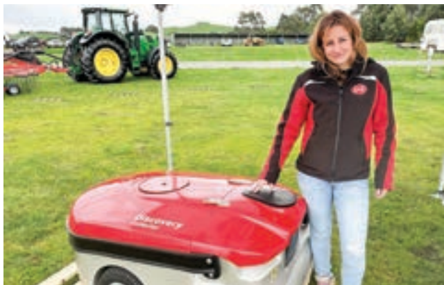
Andrea Meerwarth from Lely explains how the Lely Discovery Collector can help farmers save time and water and create better cow health by vacuuming manure on a program set by the farmer. ob48_3724
