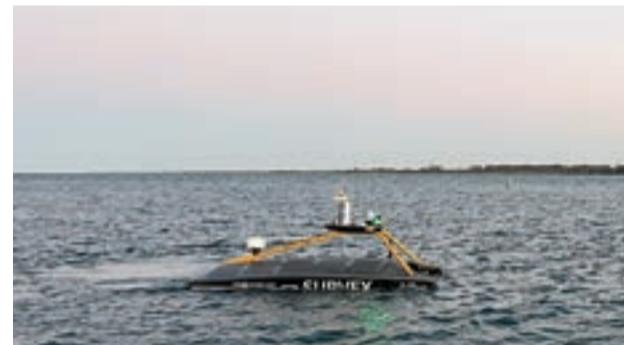
An Uncrewed Surface Vessel was launched to survey seabed conditions in Waratah Bay.
