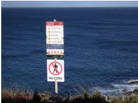
Obs 1 - Defined access sign, partly consistent with AS/NZS 2416. A review of the symbols and symbol and text height specific to viewing distance should be undertaken.
