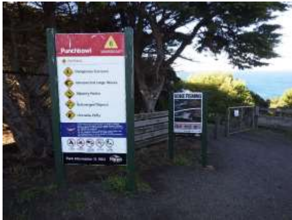
Obs 1 - Primary access sign at main entrance point. The 'No Lifesaving Service' symbol is not part of the AS/NZS 2416.1 Standard.
