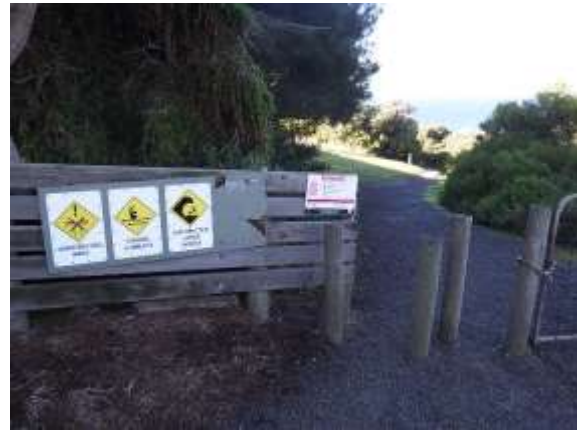
Obs 2 - Individual hazard signs used in the area in addition to several composite signs. 'Currents' and 'No Lifesaving Service' signs are not consistent with the symbols outlined in AS/NZS 2416.
