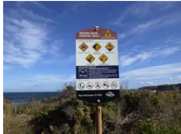
Obs 2 - Defined access sign consistent with the design intention of AS/NZS 2416. A review of the symbols and symbol and text height specific to viewing distance should be undertaken.
