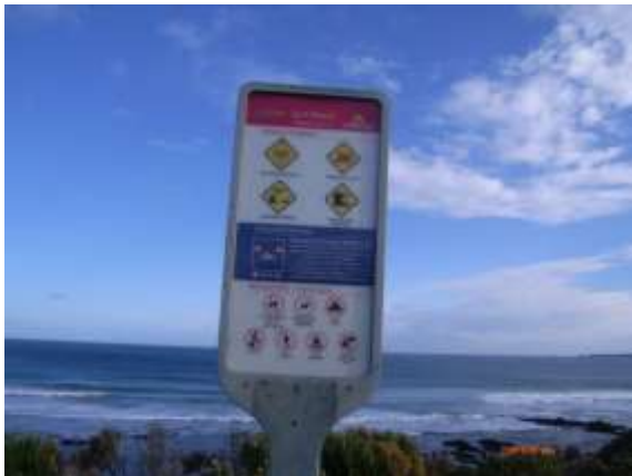
Obs 3 - Another defined access sign with the ambiguous 'No Lifesaving Service' symbol that is not part of the existing AS/NZS 2416 Standard.
