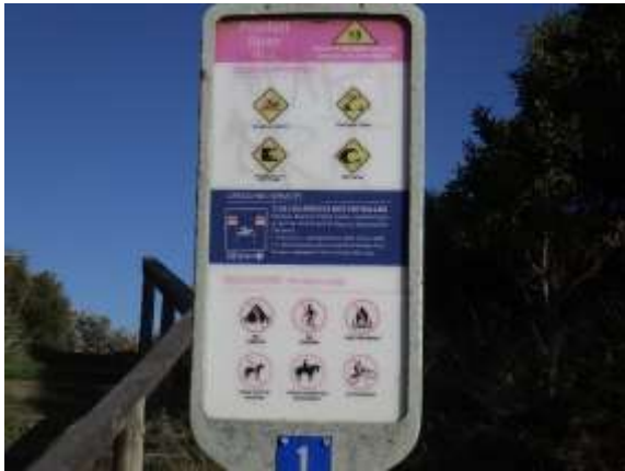
Obs 1 - Use of a defined access sign with elements that are consistent with AS/NZS 2146. Evidence of weathering and graffiti.
