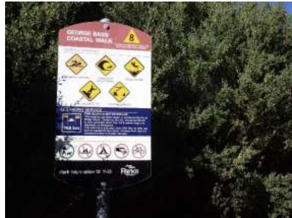
Obs 2 - Defined access sign consistent with AS/NZS 2416. A review of the symbols and symbol and text height specific to viewing distance should be undertaken.
