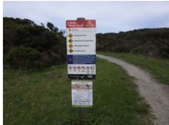
Obs 2 - Defined aquatic safety signage at site consistent with the design intention and placement application of AS/NZS 2416. Access is soil based and uneven in areas.
