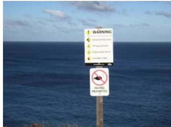
Obs 2 - Defined access sign variation that uses the 'No Lifesaving Service' symbol that is not part of the AS/NZS 2416.1 Standard. Every effort should be made to keep sign styling and symbology consistent.
