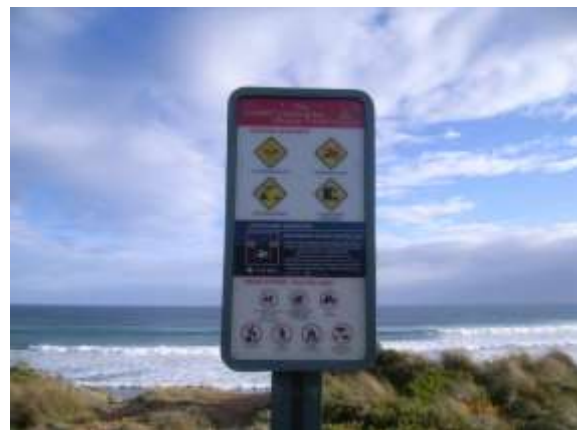
Obs 6 - Another safety sign with the 'No Lifesaving Service' symbol that is not part of the existing AS/NZS 2416 Standard. Signs should also be reviewed in terms of placement and symbol and text heights.
