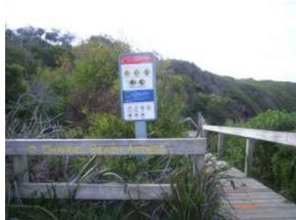
Obs 2 - Aquatic safety sign reflective of the design and application intent of AS/NZS 2416.
