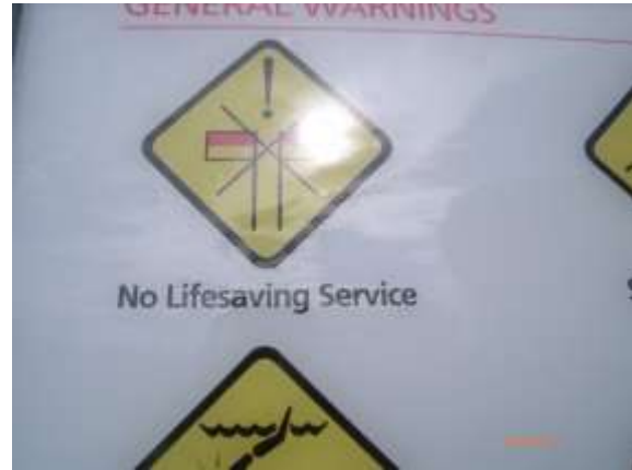
Obs 2 - Sign uses a 'No Lifesaving Service' symbol that is not found in the current AS/NZS 2416 Standard.
