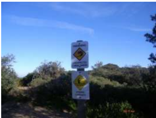
Obs 3 - Warning signs advising of large unexpected waves and strong currents. The 'Strong Currents' symbol is not consistent with the Standard.
