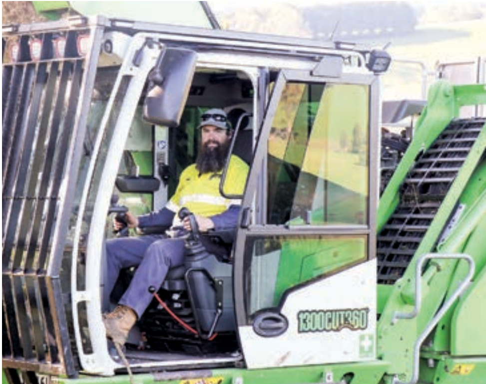
Konrad Bourn operating the Sennebogen 718 tree handler at a controlled height to cut and move dangerous limbs hanging over a shed. Z02_2822
