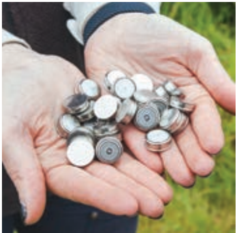
Loggers have been placed at penguin height across the Summerland Peninsula to record the temperature and humidity across different habitats.
