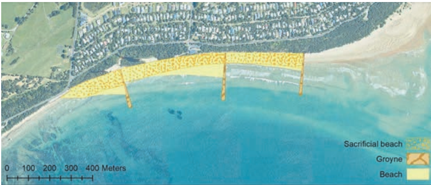
A system of beach groynes has been proposed to support the dunes which provide protection to some of the impacted residential areas.
