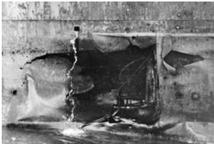
A 12-foot by 14-foot hole on the waterline under the bridge on the port side of HMAS Australia. This damage was inflicted by a Japanese Kamikaze aircraft attack on 7 January 1945. A temporary patch is covering the damage.
