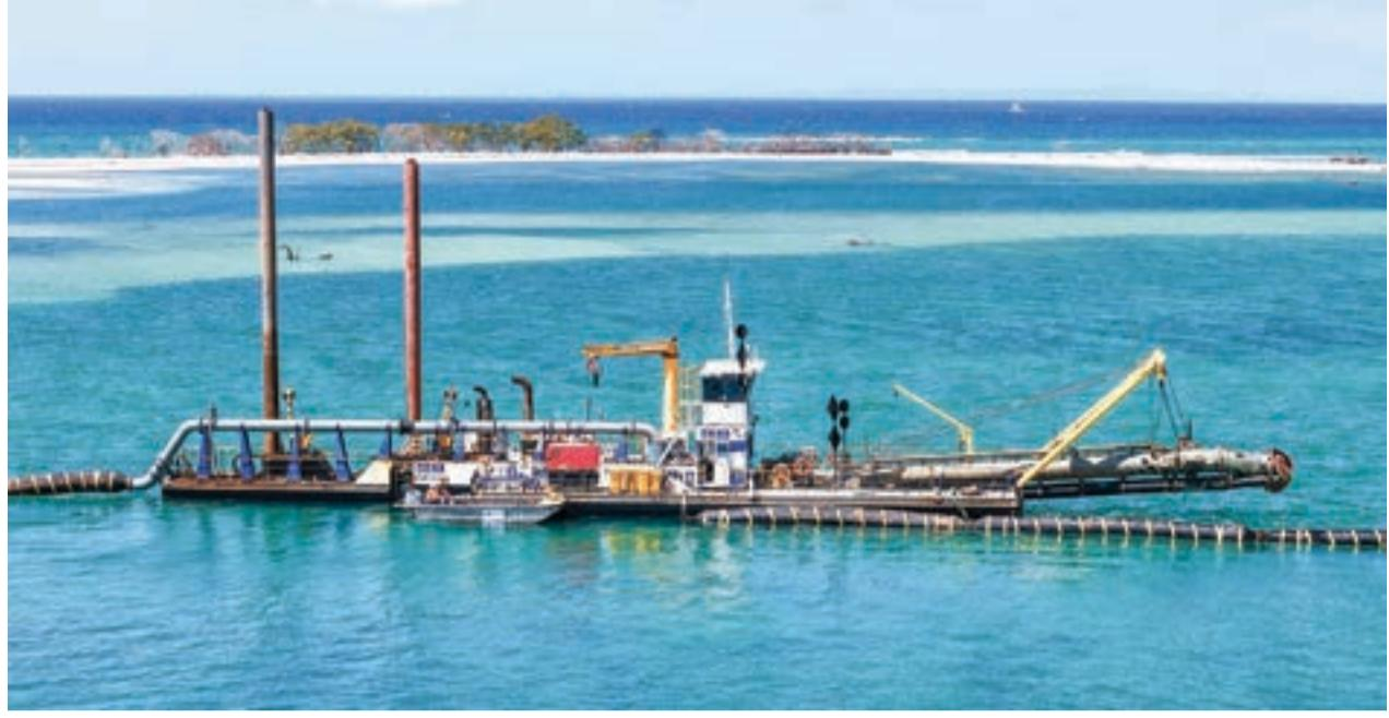
A similar but slightly smaller cutter suction dredge operated by Hall Contracting will soon be on its way to Anderson Inlet to start sand renourishment works at Inverloch.
